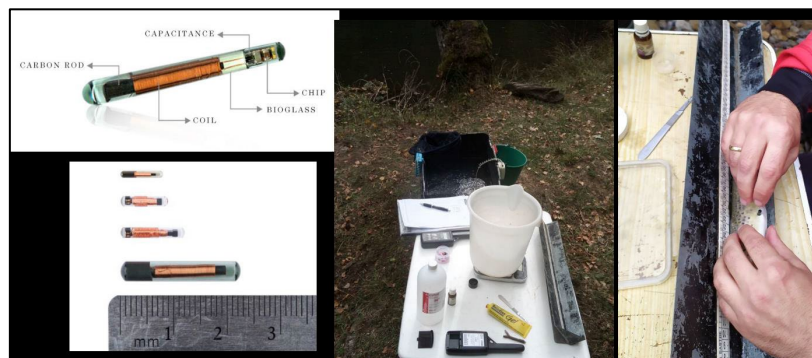
Figure 26. PIT-tags, field monitoring station and placement of the PIT in the intraperitoneal cavity of a trout.
