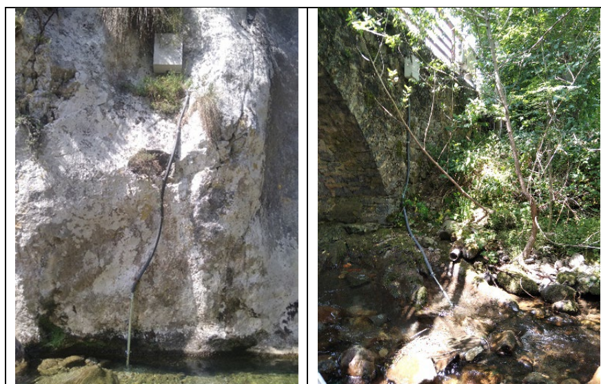
Figure 62. Gauge stations in Picos4 (Duje river) and Picos6 (Cares river; Posada de Valdeón).
